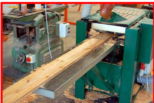
Stacking and machine edge-profiling of tongue-and-groove red cedar cladding boards, Rawnsley Woodland Products, Cornwall
