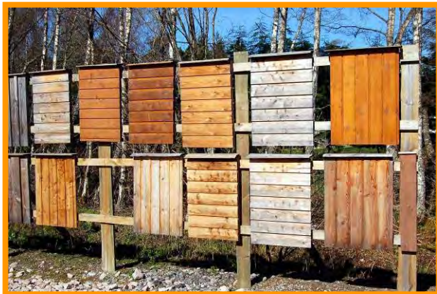
Scotlarch cladding (Russwood of Newtonmore) - trials of alternative finishes at the sawmill and as installed on NTS Culloden Battlefield Centre
