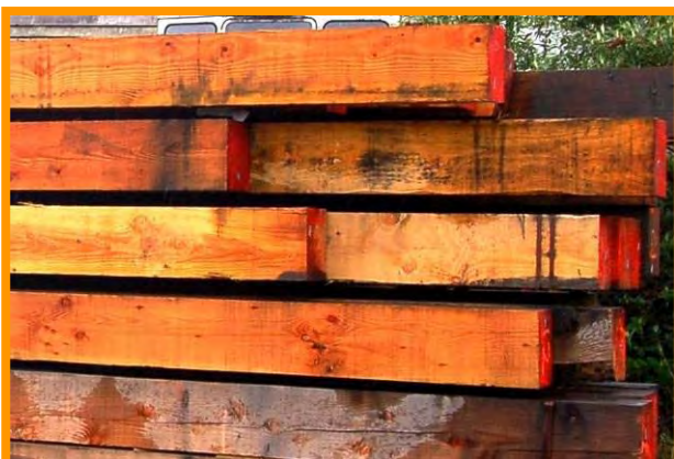
Premium larch for marine beamworks - extraction (JB Timber Ltd) and as sawn into long-length beams (Gilmour & Aitken Ltd)
