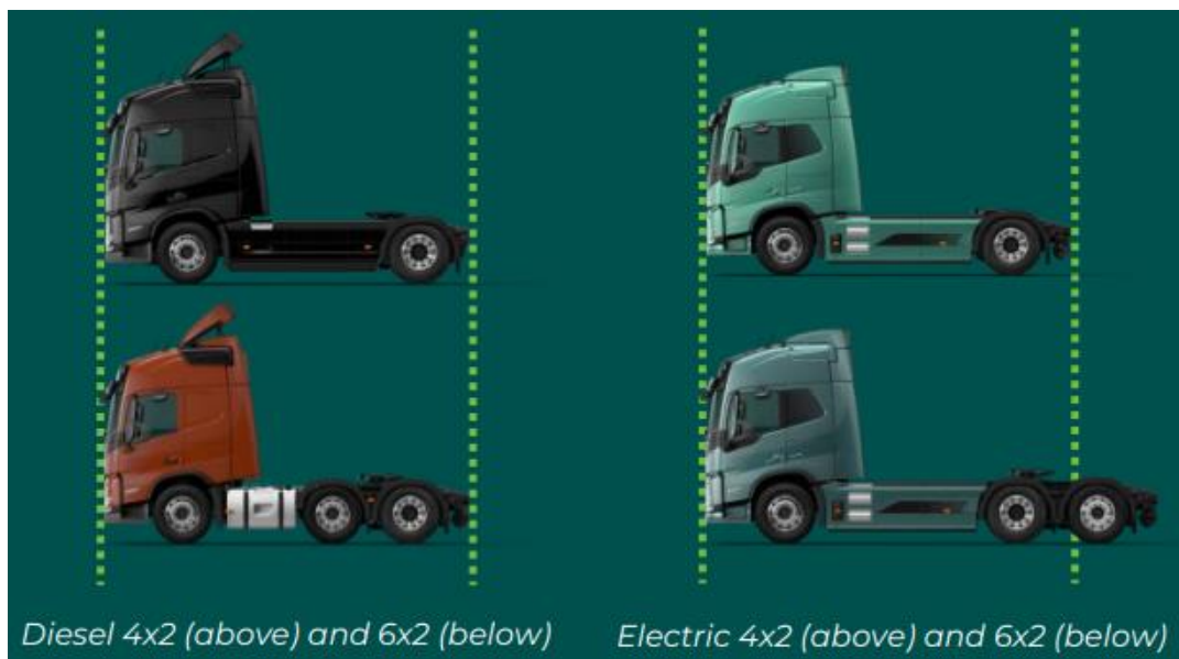
Figure 4: ICE vs EV HGV axle configurations to accommodate batteries.
