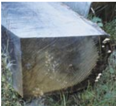
Above Sapwood in sweet chestnut log. The outer sapwood has started to decay after only a few months in a damp environment.
