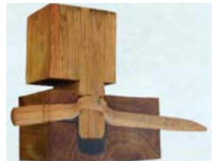
Figure AIII.2 "Freeze frame" specimen technique developed by J. Shanks at University of Bath - transparent epoxy resin is poured into the joint whilst it is still deformed under test. The specimen is sectioned after the resin has cured Photo: C.Mettem
