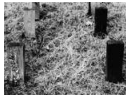
Figure 4.8 'Graveyard' tests Photo: © BRE
