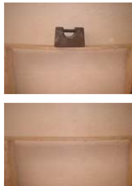
Figure 4.11 a, top: A plank of green oak, 100 mm wide by 20 mm deep, spanning 1.2 m with a central point load b, above: After six months the plank had dried out. With the load removed, a residual deflection of 19 mm remained
