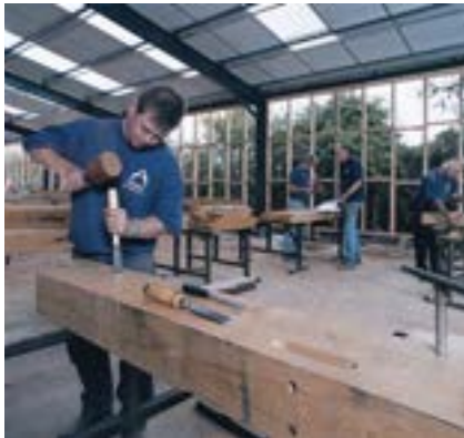
Figure 6.5 After main preparation using Hundegger equipment, green oak framing work is completed using traditional hand tools Photo: T J Crump Oakwrights
