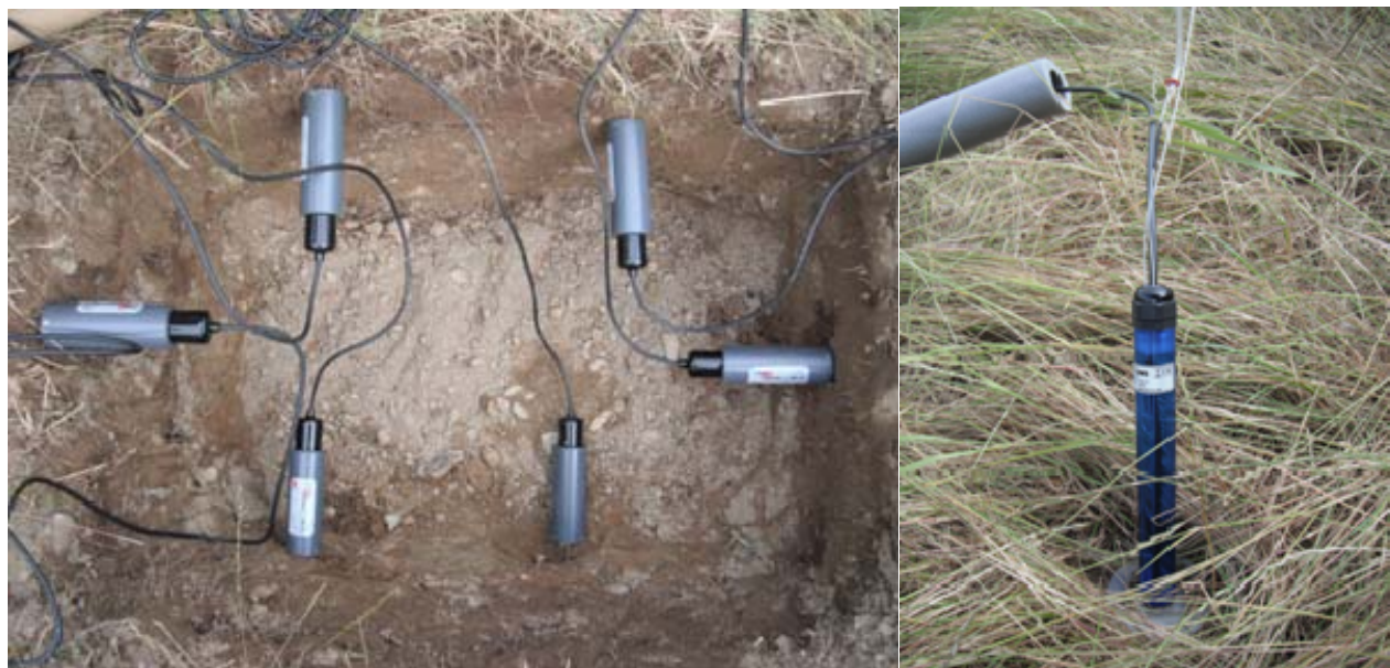
Figure 2. Soil moisture probes installed at various depths in soil profile to measure soil moisture content (left) and tensiometers to measure soil water potential.
